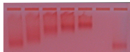
Figure 2. Formation of PBS DNA SH–gold nanocolloid complexes. The increasing shifts in the gel (lanes 1–5) illustrate that increasing the concentration of primer PBS DNA SH relative to the concentration of gold nanocolloids results in more primers attached per colloid. Lane 7 is a control containing gold nanocolloids only.
